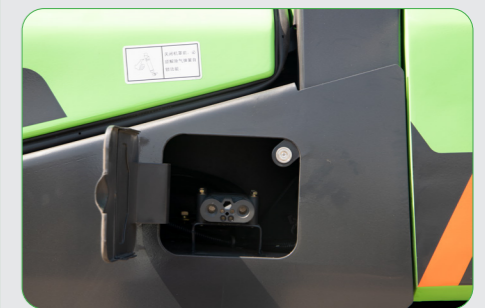
Configure an External Charger • External 65A charger, input voltage three-phase 380V; optional 100A or 150A charger to achieve fast charging
