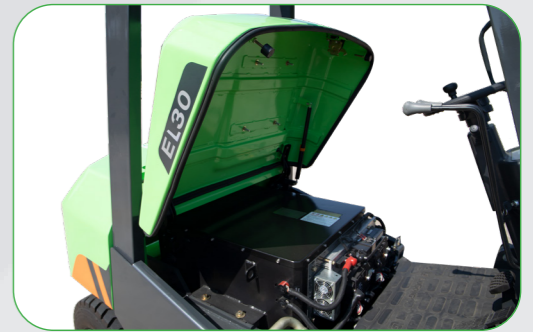
Large Angle Opening of Engine Hood • The opening angle of the hood is large, and the battery, electric control, and motor can be accessed directly after opening the hood, which makes maintenance more convenient Removing Floor with Tool-free • Simple operation, saving time and labor for routine maintenance
