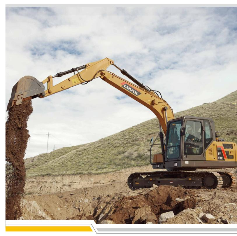
Rated Power Operating Weight Bucket Capacity 72.7kW/2200rpm 13850kg 0.53m<sup>3</sup>
